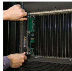
The Network I/O enclosure provides X.25 and X.29 communication
